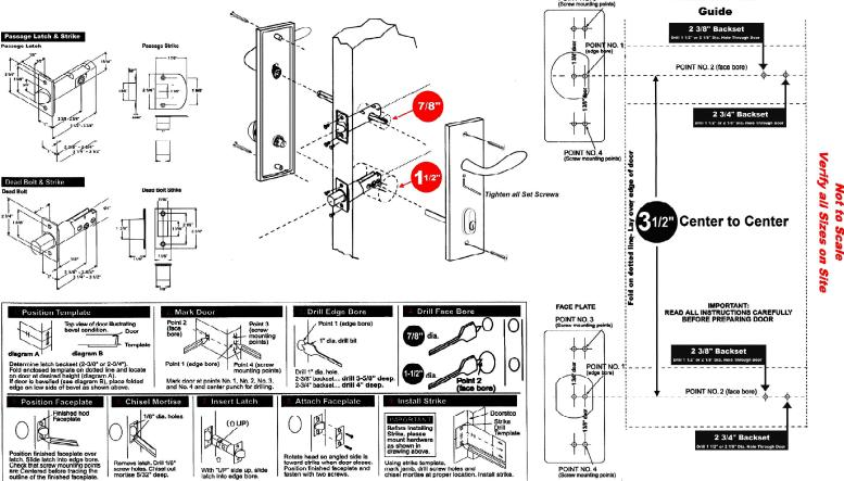
NOTE: Check to ensure face plate does not restrict free movement of the latch head. Repeat instruction 1 - 9 for latch bolt , Install trim,
